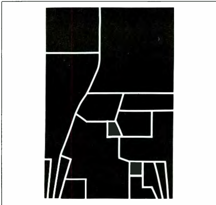
Fig. 3. Actual-size etching-and-drilling guide for printed-circuit board.
