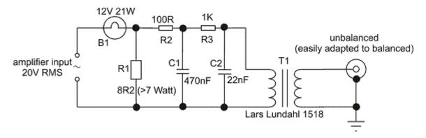
The circuit for the "Hot Lamp" speaker-simulator is given in figure 1. It is a "cinch" to build: it is so simple that a PCB is not required. (The photo' below illustrates the working prototype).
