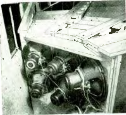
Fig. 2—How the six speakers are mounted.
