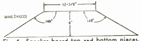
Fig. 4—Speaker board top and bottom pieces.
