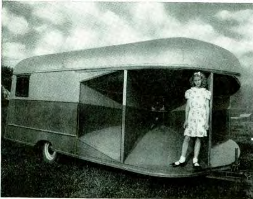
Occupying the entire trailer front end, this horn is limited only by the power feeding it.
