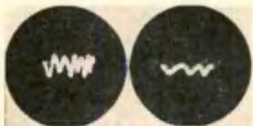
Fig. 12. Acoustic output at 32 cps. Although slightly lower in output, the R-J—at the right—is still fundamental in character.
