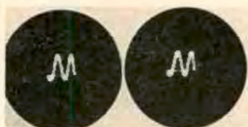
Fig. 9. Acoustic output at 55 cps. Left, bass reflex; right, R-J.
