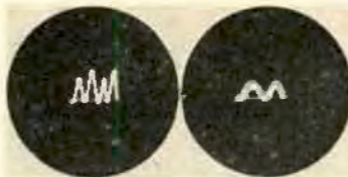
Fig. 11. Acoustic output at 44 cps. Output from bass reflex is seen to be almost 100 per cent harmonic, due to frequency doubling.
