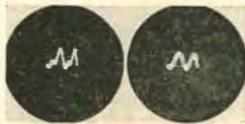
Fig. 10. Acoustic output at 48 cps. Note beginning of frequency doubling from the bass reflex at the left; the R-J is still fundamental.
