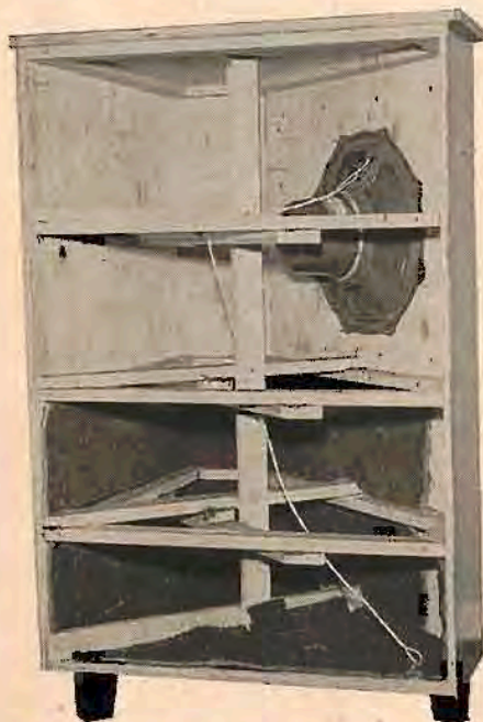
Fig. 3. Internal view with one back panel removed to show cross bracing and unsymmetrical mounting of the speaker. Also note start of Ozite lining in lower part of cabinet.
