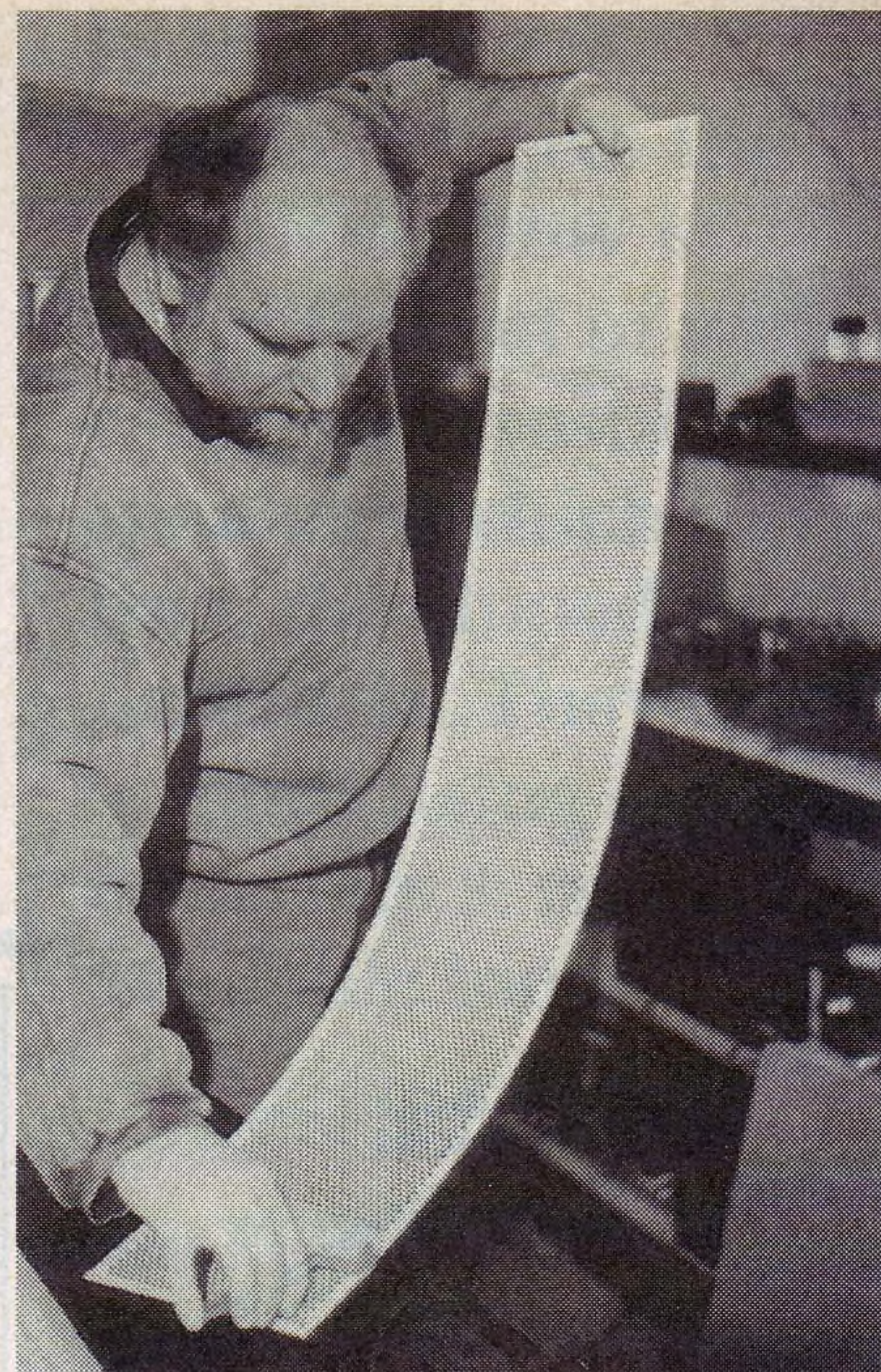
Adhesive is applied to the perforated grid with the aid of a smaller paint roller, before the grid is attached to its matrix panel.
