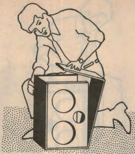
Although illustrating a somewhat larger enclosure, the diagram emphasises the extreme simplicity of the fold-around method of construction.
