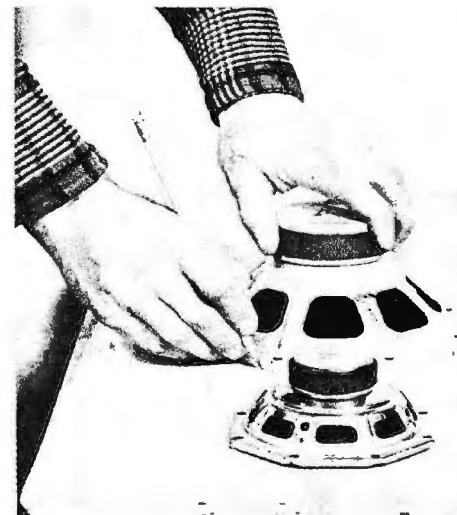
Fig. 2. Use speakers as patterns for octagonal cutouts on sides.
