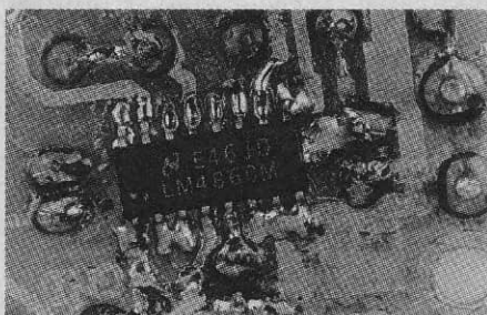
The LM4860 IC (IC1) is mounted on the copper side of the PC board as shown here. Use a fine-tipped soldering iron for this job & make sure that the device is correctly oriented.
