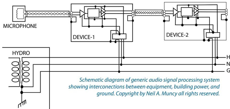
*Schematic diagram of generic audio signal processing system showing interconnections between equipment, building power, and ground. Copyright by Neil A. Muncy all rights reserved.*
