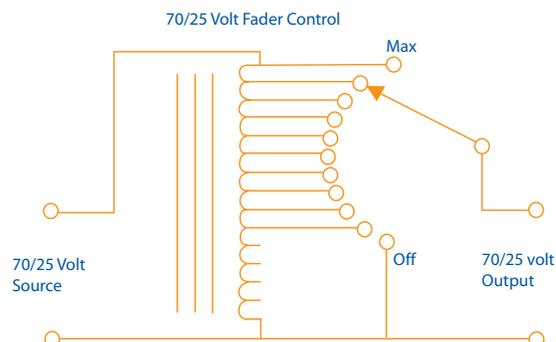
These controls will reduce the volume to the systems that they feed, still at 70 (25)-V. Although not usually done, use of series/parallel circuits can still be used on the 8-ohm output side of the transformer to limit the number of transformers used in low power situations.
