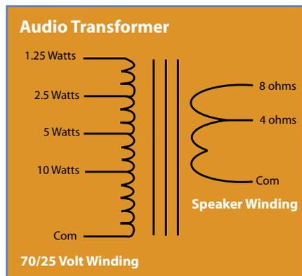
The 70(25)-V line from the amplifier is applied to the input of the transformer. The input selected is based on the maximum power needed from the speaker. Each speaker location comes from this same 70(25) volt line source (in parallel). The sum of the power setting of all transformers used should be less than the maximum power of the amplifier.
