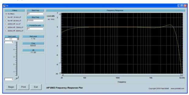
...the peaking at HF can be adjusted by changing the RC loading on the transformer secondary.
