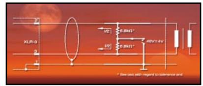
Fig. 1. A standard 48 Volt phantom powering arrangement (console or microphone preamplifier shown with input transformer).
