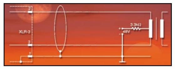
Fig. 2. An alternative 48 Volt phantom powering arrangement with centre-tapped input transformer.
