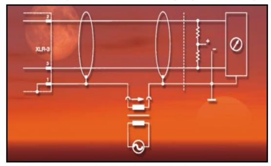
Fig. 3. A circuit for testing the susceptibility of a microphone to induced interference.
