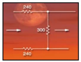
Fig. 4. Balanced resistive pad, suitable for use with phantom-powered microphones.
