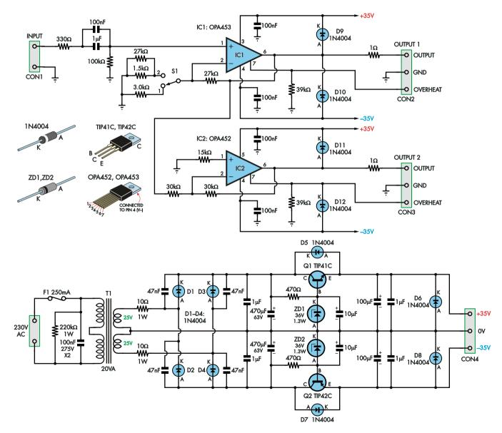
$30k\Omega$  resistor. The gain of IC2 is set to -1 due to the use of two  $30k\Omega$  feedback resistors, with a  $15k\Omega$  resistor tying pin
