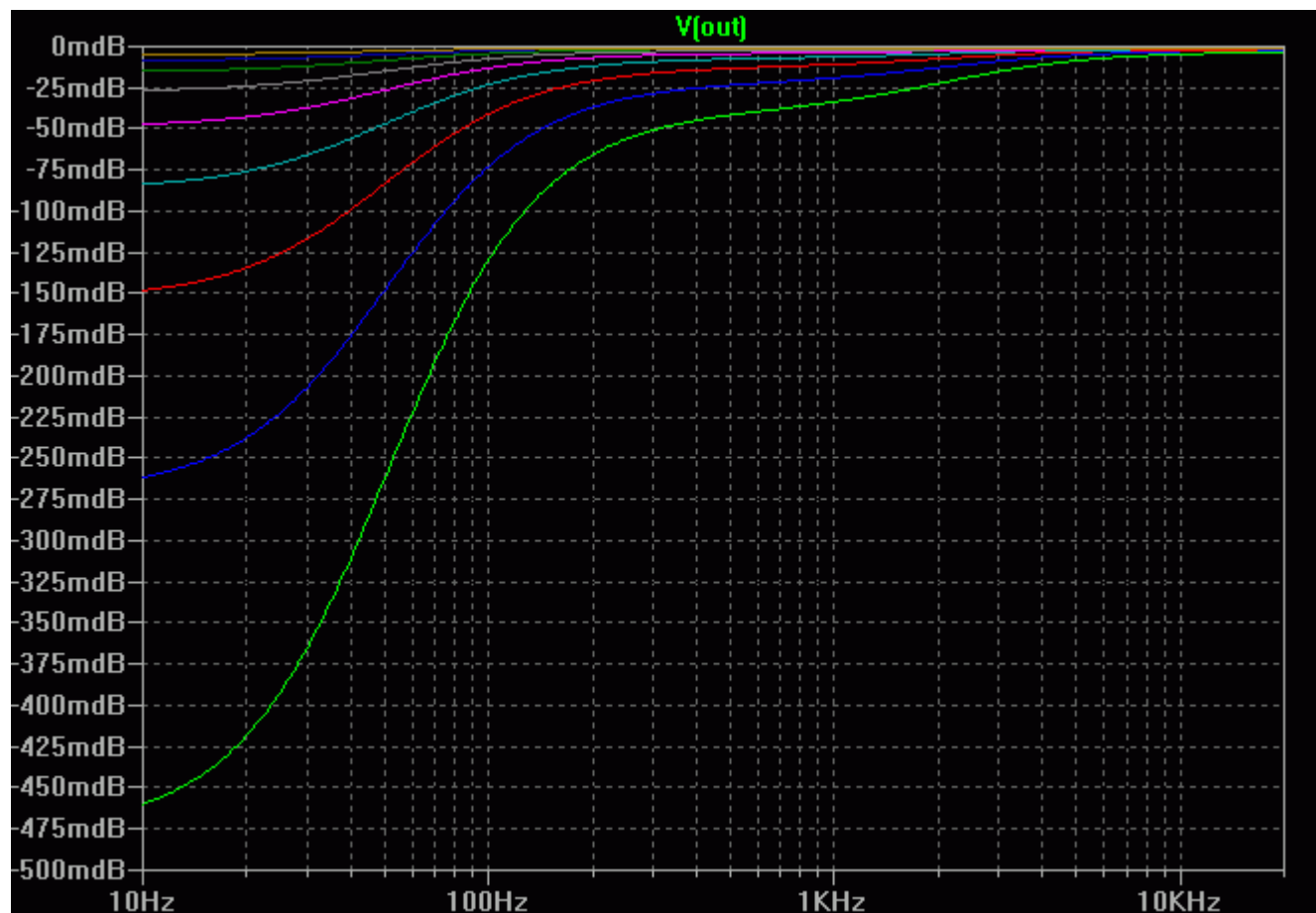
Figure 7. Equalization Error From Finite DC Open-loop Gain
