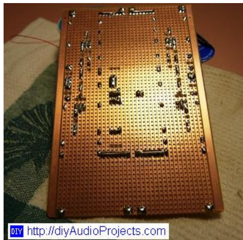
Photograph 4: DIY JFET RIAA Preamp on Stripboard
