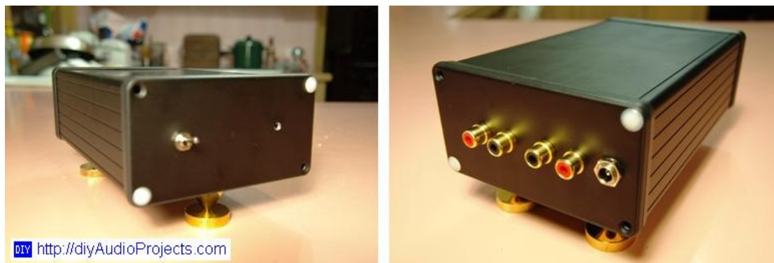
Photograph 5: DIY JFET RIAA Preamp in Hammond Enclosure
