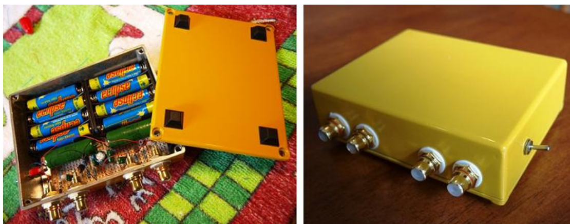
Photograph 7: DIY Le Pacific MC PrePre in Aluminum Enclosure
