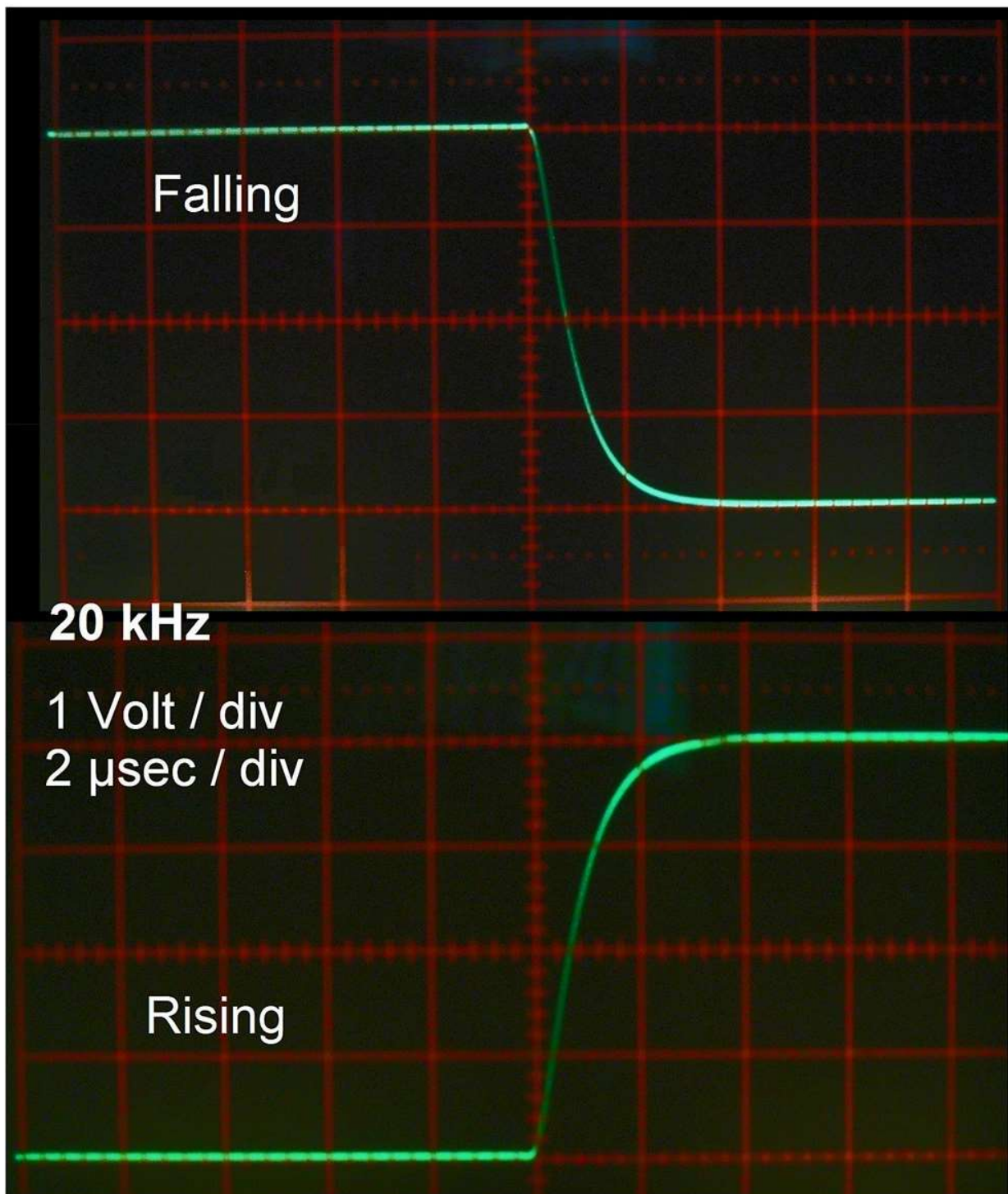
Photo 7: The response of Inverse RIAA network and the preamplifier on a 20-kHz square wave is shown.
