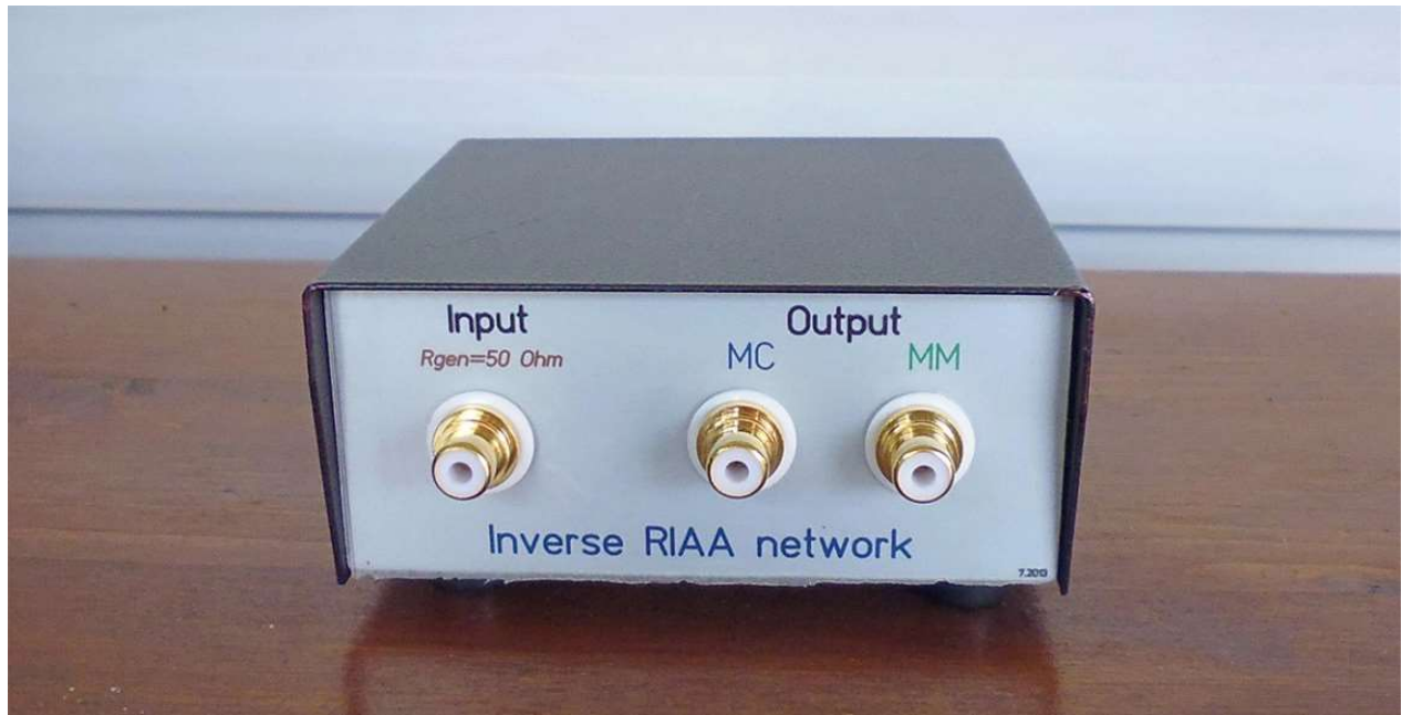
Photo 6: This enclosure contains the inverse RIAA network that I used for the measurements.
