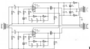
Here the RIAA stereo preamplifier classic version based on NE5534. This setting is intended for use with a vinyl turntable equipped with an analog output (RCA). It provides the dual function of pre-amplification and RIAA correction. This RIAA pre amp circuit is suitable for MM cells (Moving Magnet), and is not suitable for cell MC (Moving Coil). It is slightly more efficient than "RIAA stereo preamplifier classic version, based on the NE5532".
