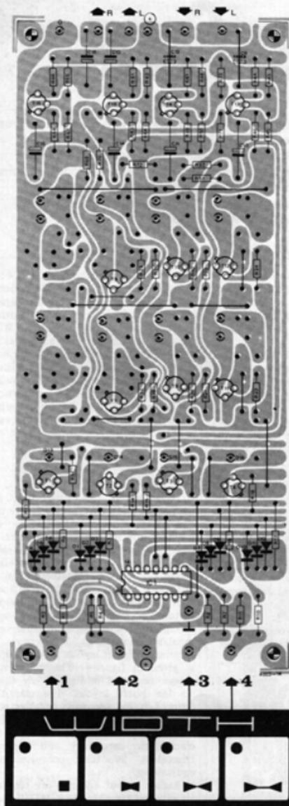
Figure 14. Component layout for the stereo width control (figure 9).
