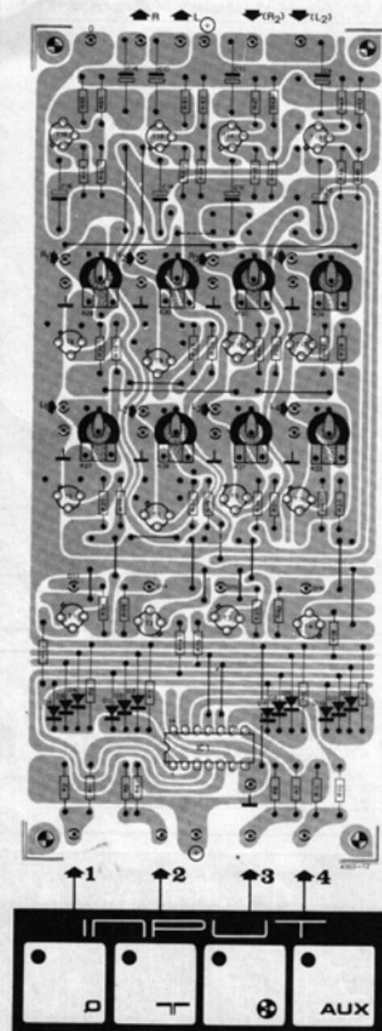
Figure 12. Component layout for the input selector (figure 3).
