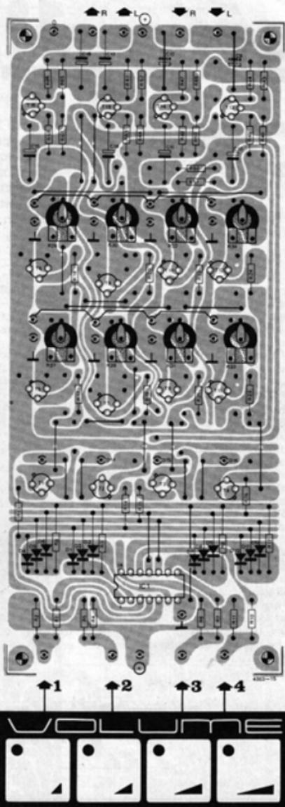
Figure 15. Component layout for the volume control (figure 10).
