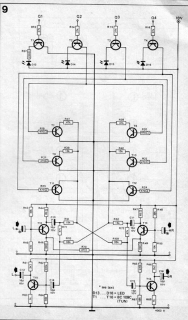
Figure 4. The tone control unit. The four positions give bass boost, middle lift (presence), flat response and treble cut respectively.
