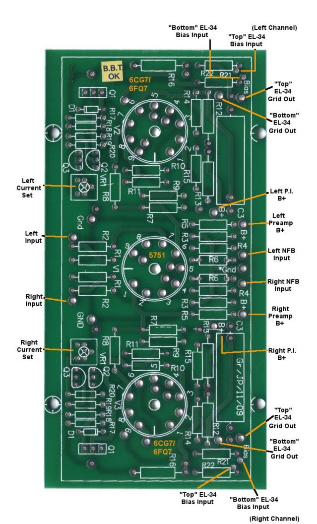
Obeying this keeps the proper phase of the NFB. This is very important as if the grid drive is reversed, it will turn your ST-70 into a power oscillator damaging not only your amplifier, but your speakers and likely your hearing in the process.
