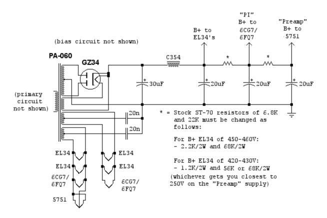
In our R&D of this board, it was found that the output voltage of the stock PA-060 varied pretty significantly depending on line voltage. At our facility, line voltage is almost constant at 125VAC with a measured high of 126.3V and low of 123V. Therefore our PA-060 was putting out an incredible amount of voltage and we used 2.2K, 2W and 68K, 2W.
