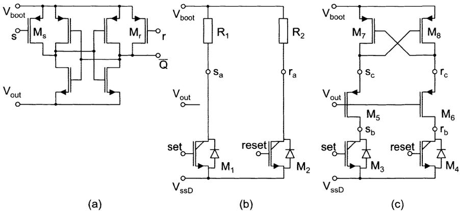
Figure 17. Levelshifting (a) latch (b) simple levelshifter (c) current efficient levelshifter
