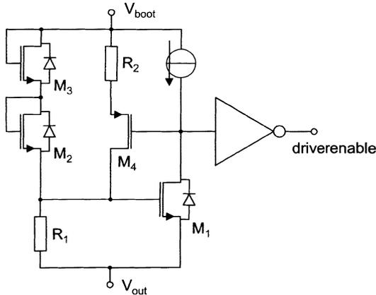
Figure 14. Highside driver undervoltage protection
