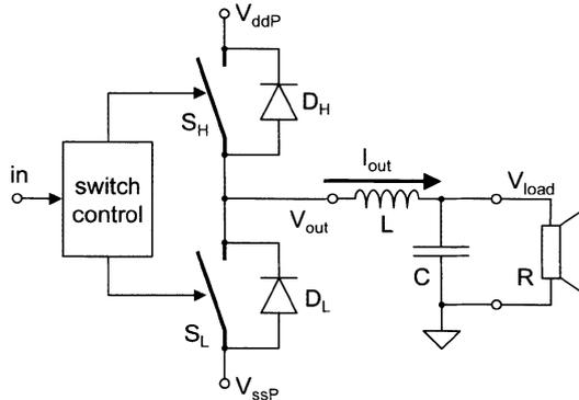
Figure 1. Class-D output stage
