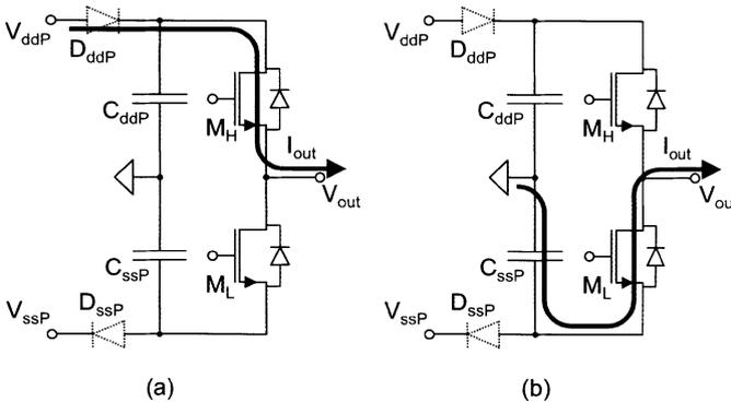
Figure 9. Supply pumping (a) sourcing current from positive supply (b) charging decoupling capacitor negative supply
