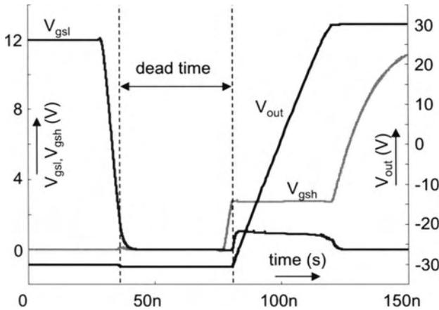
Figure 11. Voltage transients with  $I_{out}=0$
