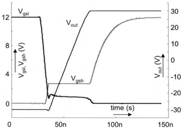
Figure 15. Zero dead time voltage transients
