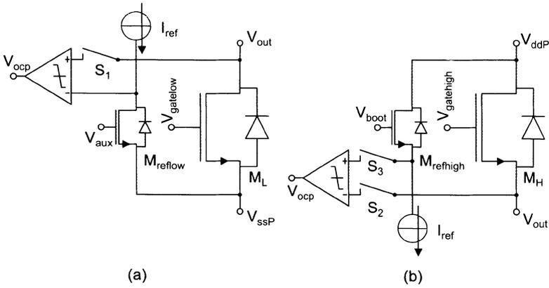
Figure 8. Overcurrent detection (a) lowside (b) highside
