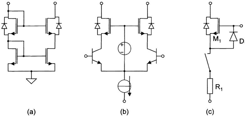
Figure 4. High voltage circuit techniques (a) current mirror cascode (b) differential pair cascode (c) gate-source clamp
