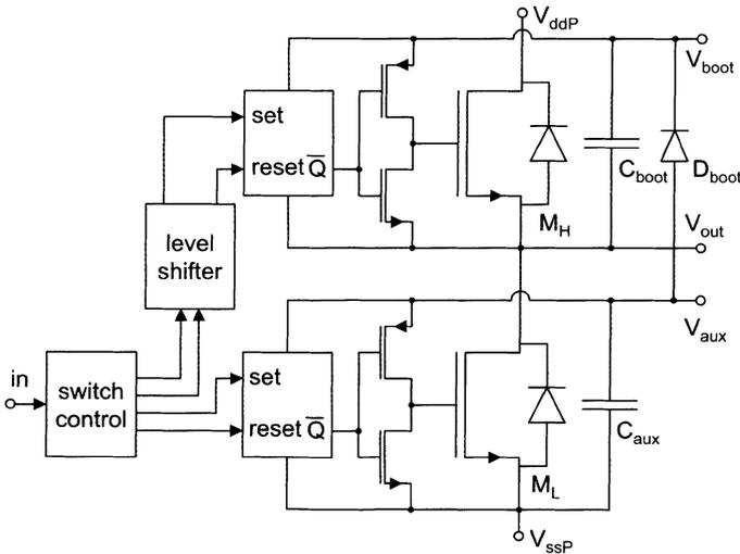
Figure 3. Class-D output stage with nDMOS power transistors
