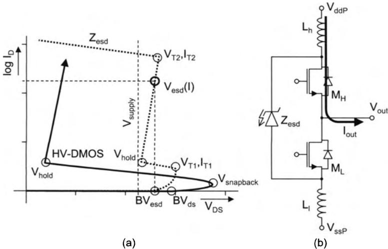
Figure 5. High current switching (a) breakdown characteristics (b) parasitic inductance.
