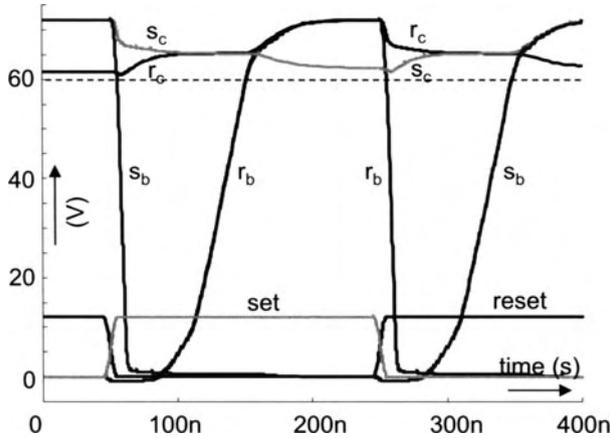
Figure 18. Voltage transients in level shifter
