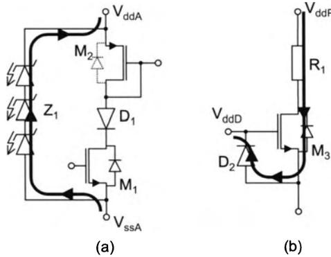
Figure 7. ESD measures (a) blocking reverse current paths (b) limit breakdown currents
