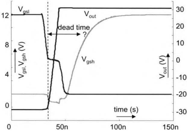
Figure 13. Voltage transients with  $I_{out}=10A$
