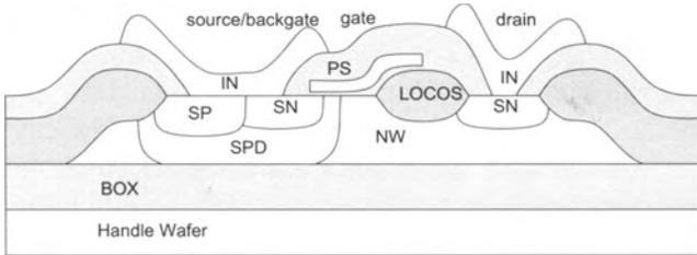
Figure 2. Cross-section of a 60V N-DMOS in A-BCD
