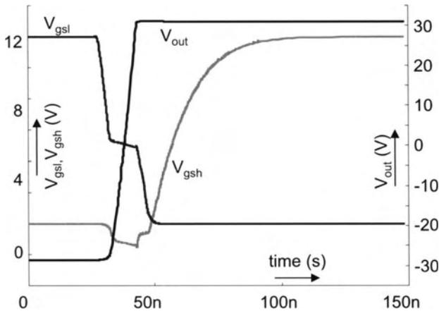
Figure 16. Zero dead time voltage transients with  $I_{out}=10A$
