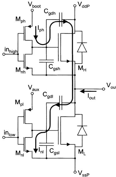
Figure 10. Simplified Class-D Powerstage
