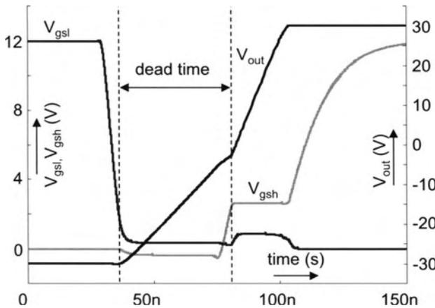
Figure 12. Voltage transients with  $I_{out}=100mA$
