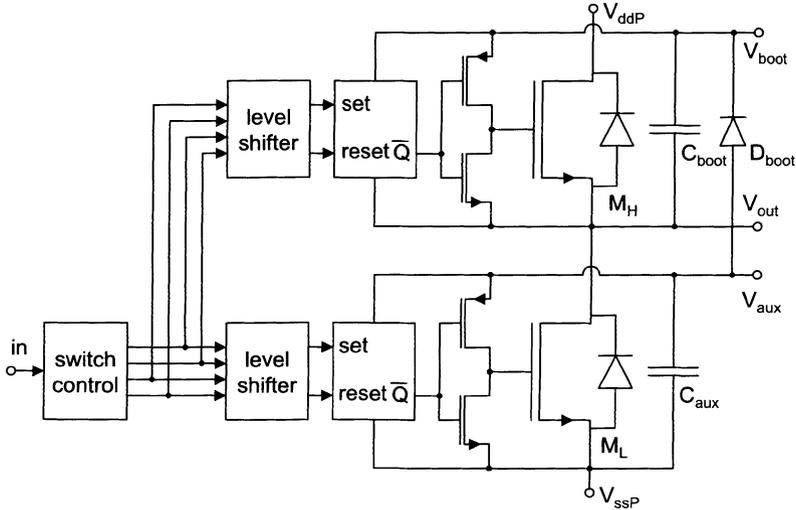
Figure 21. Delay matching highside and lowside
