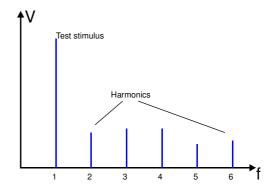
This renders THD measurement impractical at higher frequencies. For example, if we want to do a THD test at 20kHz, one needs a 60kHz measurement bandwidth just to capture the second and third harmonic, let alone any higher-order nonlinearities.
