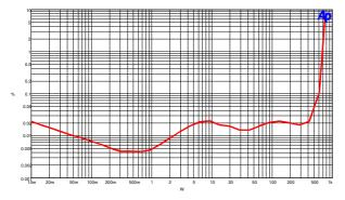
Slew rate distortion will become noticeable only when the slew rate is 70% of the limiting value. This happens at (70%\*35kHz=) 20kHz and even then only at full power (when "normal" distortion is already higher). So, slew rate distortion is completely swamped by level-dependent distortion up to a full scale 20kHz input. I think that's reasonable.
