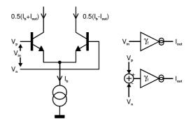
The transfer function shows differential output current vs differential input voltage. The transconductance is the slope of the transfer function.
