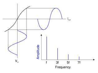
If one wishes, the transfer function can be reconstructed based on the amplitude and phase of the distortion components. A single THD spectrum will do to characterise **fully** the distortion mechanism. Next, the same non-linearity is confronted with two sinusoidal inputs.
