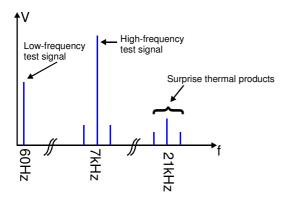
In both cases, the large difference in loop gain between high and low frequencies accounts for the discrepancies between THD and IMD figures. When doing tests on amplifiers with large DC loop gains the most directly useful distortion measurements are always the ones that put the relevant distortion products at higher (but still sub-20kHz) frequencies to keep them from being suppressed beyond measurement by the control loop. Sometimes, the best test is a THD measurement, sometimes it's IMD.
