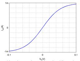
The amplifier slew-rate limits when the differential output current equals bias current i.e. when one of the two transistors is completely cut off.
