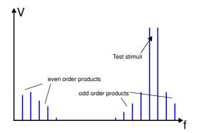
Suddenly the 20kHz audio band is wide enough to hold in all 38 distortion components (not counting the two stimuli). In a "memory-free" non-linearity, the individual components that we find in the IMD test are the same as the ones found in a simple single-tone test (with the same peak amplitude).
