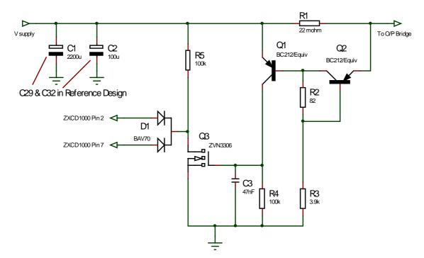
The recommended solution for short circuit protection senses the current in a small resistor (R1 - 22 milli-ohm) which is fitted between the existing reservoir capacitors (C1 & C2) and the Output Bridge formed by the four FETs.
