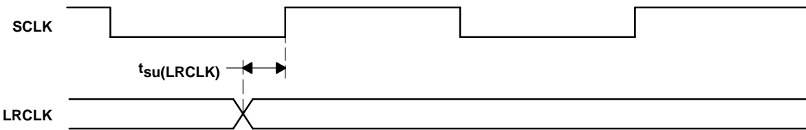
Figure 12. Right, Left, and IIS Serial Mode Timing Requirement
