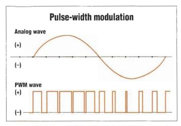
Pulse-width modulation substitutes the duty cycle of a switched waveform for the value of an analog voltage. The chart shows typical output pulse widths for different points along the sine wave. The PWM wave possesses a 50% duty cycle without an output signal and is at least 10× the frequency of the highest sinewave output frequency.
