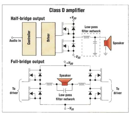
Class D amplifiers possess outputs similar to those found on servomotorcontrol systems with a speaker taking the place of the motor. Pulsewidth-modulation techniques control the power delivered to the speaker while the output transistors cycle between full-on and full-off modes at a high switching rate.
