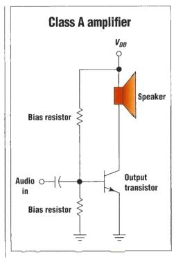
Class A amplifiers bias their output to the middle of their linear region. The amplifier continuously draws current even in its quiescent state. While its theoretical efficiency is 25%, it rarely exceeds 20% and is usually far less efficient in actual use.
