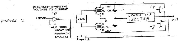
We decided to concentrate on class g assemblies, wherein we could smoothly bring additional output devices into play, taking advantage of their added dissipation capability--and surprisingly, also resulting in a simpler system.
