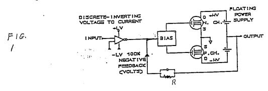
Trans\*nova employs a novel cooperation between voltage feedback, fed through the feedback resistor, and signal current from the driver stage. The result is unexpected and very desirable--an output stage with 100% negative (voltage) feedback, with no loss of voltage gain. Most of the output voltage signal trying to return through the feedback resistor is canceled by the subtractive voltage drop in the resistor caused by the drive current. Such a circuit point is called a node.
