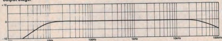
The measured frequency response of the amplifier (single module). Roll-off points are defined by the input filter (low end) and output compensation network (high end).
