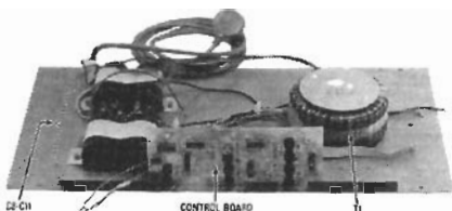
FIG. 9—THE LARGE TOROIDAL TRANSFORMER and filter capacitors provide low-ripple \pm 65 -volt outputs.
