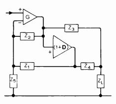
in which the class A amplifier is assumed linear with gain G, the current-dumpers unity gain with distortion (1 + D), and both amplifiers assumed to have zero output impedance.
