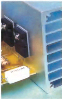
Although featuring a different amplifier module, this picture shows the vertical mounting method for the output and driver transistors.
