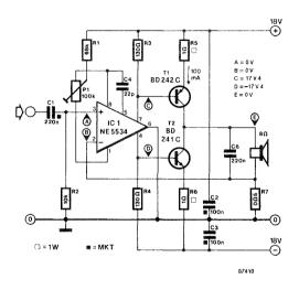
is created by feeding this reference voltage to the inverting input of IC<sub>1</sub>. The overall amplification of the circuit depends on the ratio of the loudspeaker's impedance, ZL, to the value of R<sub>7</sub>. In the present case the amplification is 16 times  $(Z_L/R_7 = 8/0.5 =$ 16).
