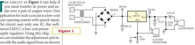
A novel circuit uses the adjustment pin of a regulator IC to provide audio amplification.
