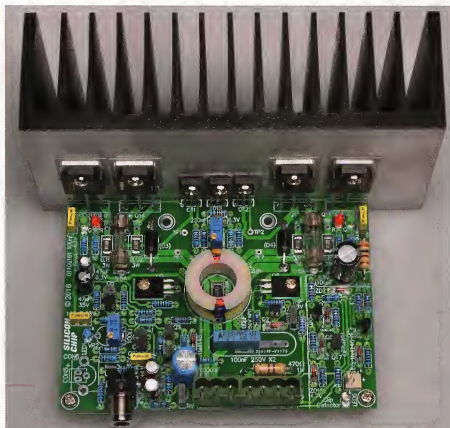
Spot the five surface-mount 3W resistors. Four are the emitter resistors for the output transistors and the fifth is inside the output inductor.
