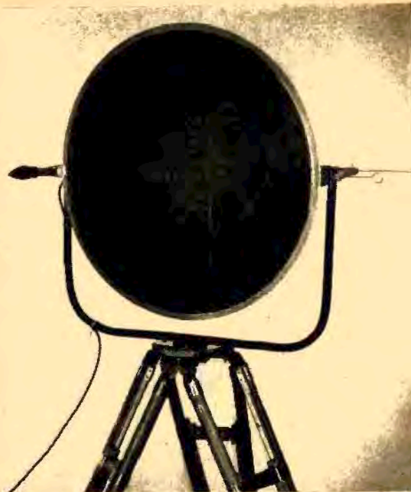
Fig. 4. Rear detail view of the parabolic microphone.
