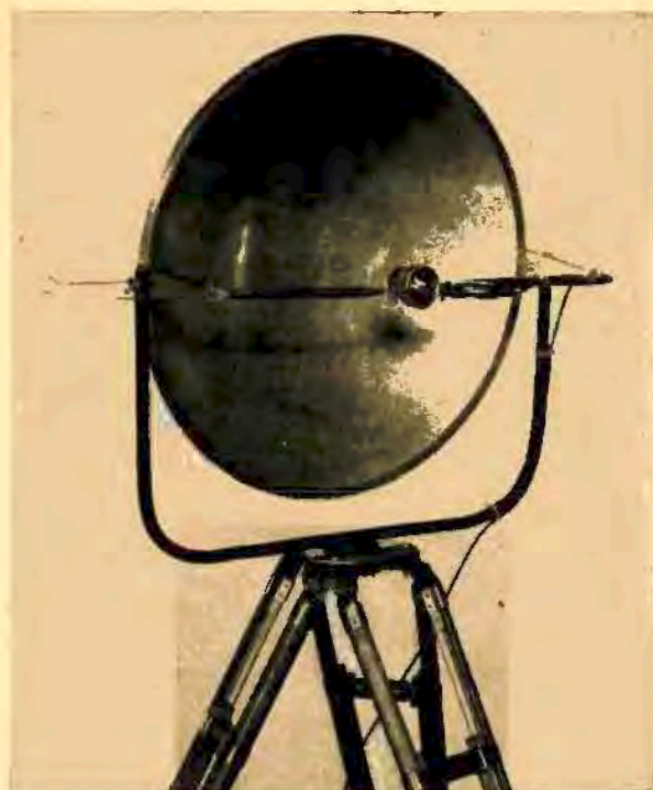
Fig. 3. Front detail view of the parabolic microphone.
