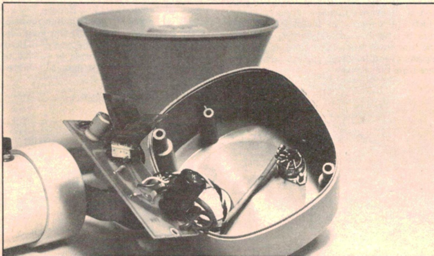
Insides out. The amplifier board mounts inside the rear cover of the Benelec 8-224 horn.
