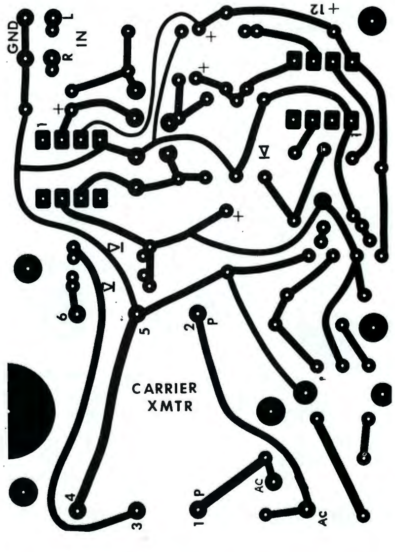
Fig. 5. Etching and drilling guide for the transmitter are shown above (A). Component placement for standard transmitter is at left (B). If pre-emphasis is used, the component placement at right is necessary (c).
