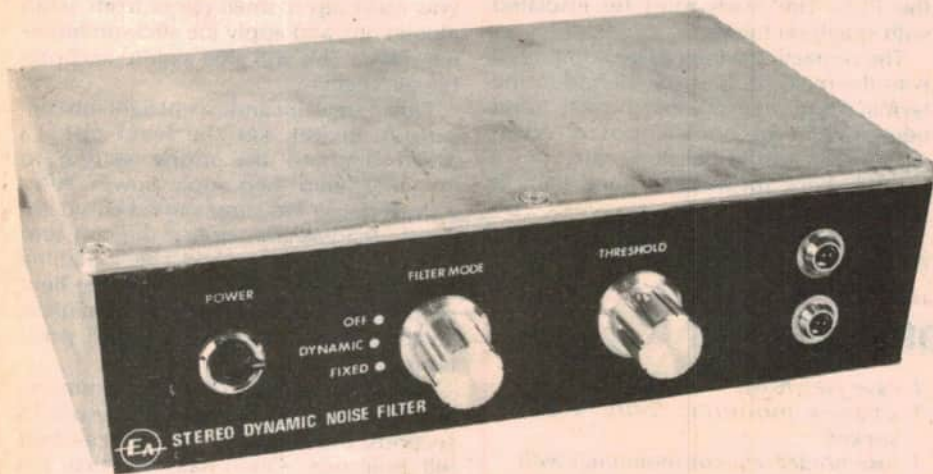
High level signals switch the filter circuits out and extinguish the two LED indicators.
