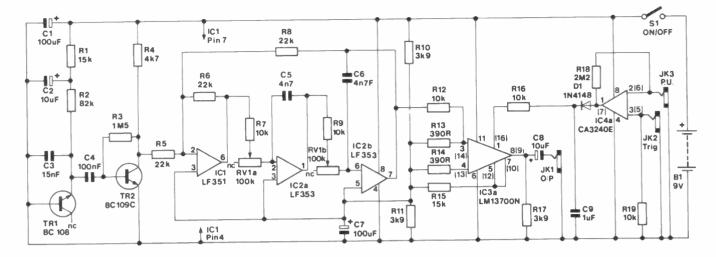
lowpass filtering that prevents the final output from having an excessive high frequency content.
