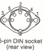
5-pin DIN socket (rear view)
