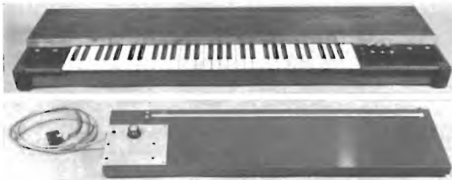
Fig. 6. (Top) Keyboard controller. Although the keyboard itself is a standard organ keyboard, the control-voltage output may be employed to control musical parameters other than the pitch. (Bottom) Linear controller. The musician slides his finger along the taut band to determine the control-voltage output.
