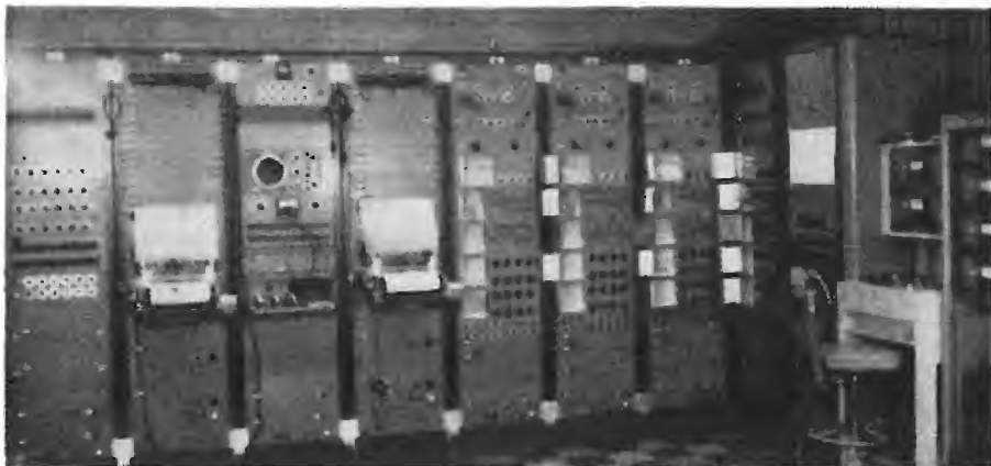
Fig. 10. The RCA synthesizer, located at the Columbia-Princeton Electronic Music Center. The rolls of paper at the center of the photograph are employed to program the entire instrument.
