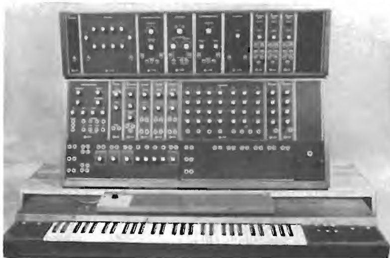
Fig. 8. The Moog Synthesizer II shown below is an audio-signal generating, processing, and controlling facility for electronic-music composition. The keyboard controller and the linear controller just above it permit control of the circuits by composer.
