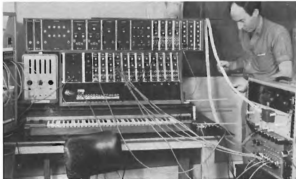
Composer Emmanuel Ghent in the studio of the Independent Electronic Music Center. The paper-tape reader at the right is being used to program the voltage-controlled instruments at the center. The frequency counter, which is located at the left, is employed to check on the accuracy of the program that is used.
