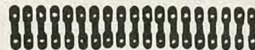
FIG. 19—FOIL PATTERN FOR HEADER STRIPS. The length of the board can be made as long or short as needed.
