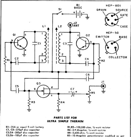
C7—10uF, 15 volt electroytic capacitor L1,L2-Loopstick (Lafayette 32-41080) Q1,Q2—HEP-50 or 2N706 transistor (Motorola) Q3-HEP-801 N-channel junction field-effect transistor (Motorola)
