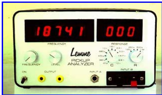
Fig.9. The "Pickup Analyzer" © - the first commercially available measuring instrument for the frequency response of magnetic pickups.
