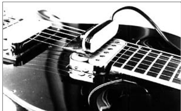
Fig.8. A transmitting coil radiates its magnetic AC field into the pickup coils. So you can measure the frequency response easily
