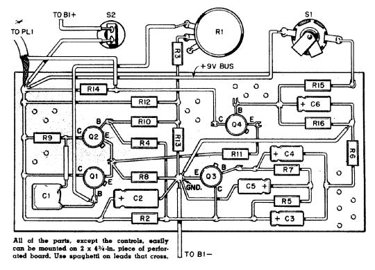
nected to the base of Q4 is a charge-storage capacitor (C6) and discharge resistor R16.
