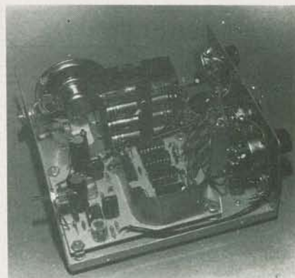
FIG. 6—AMPLIFIER SHIELD is clearly visible in photo of completed unit. Also note battery pack and vertical mounting of some diodes and resistors.
