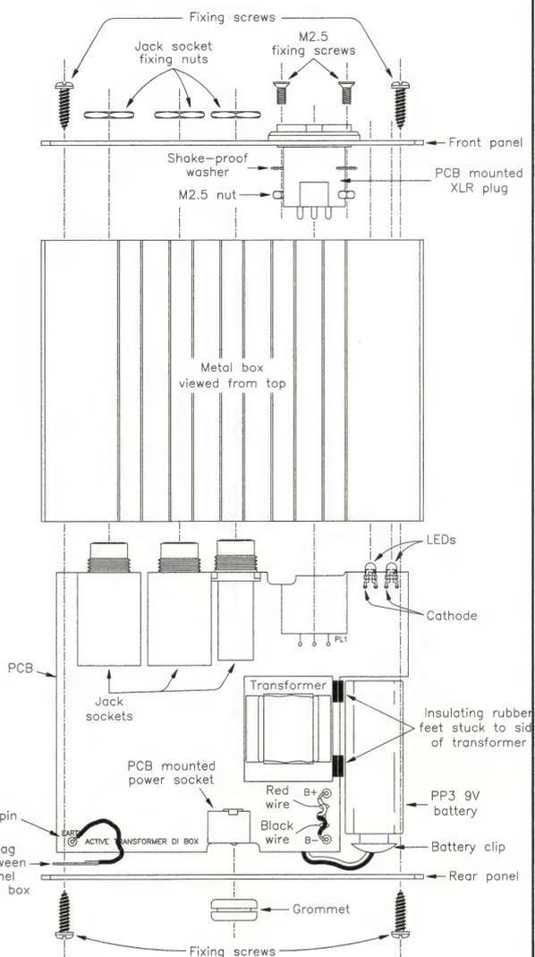
Figure 4. Exploded assembly diagram.
