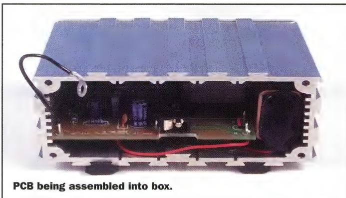
PCB being assembled into box.
