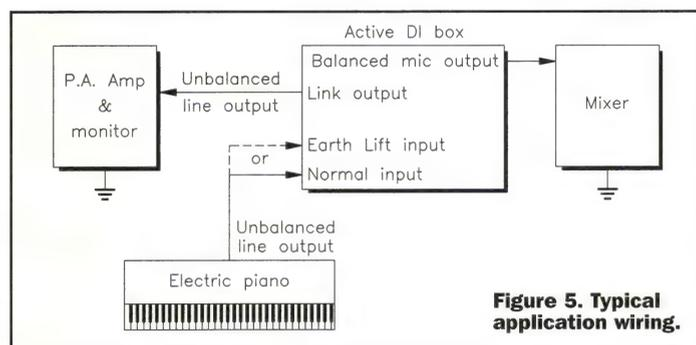
Figure 5. Typical application wiring.
