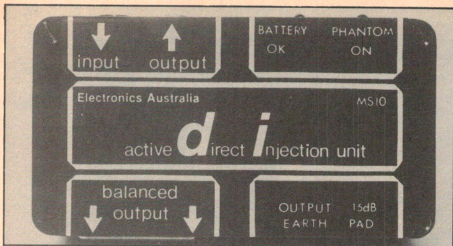
The Scotchcal front panel was trimmed to allow easy access to the box lid screws, although the battery rarely requires replacement. The actual size artwork is shown below.
