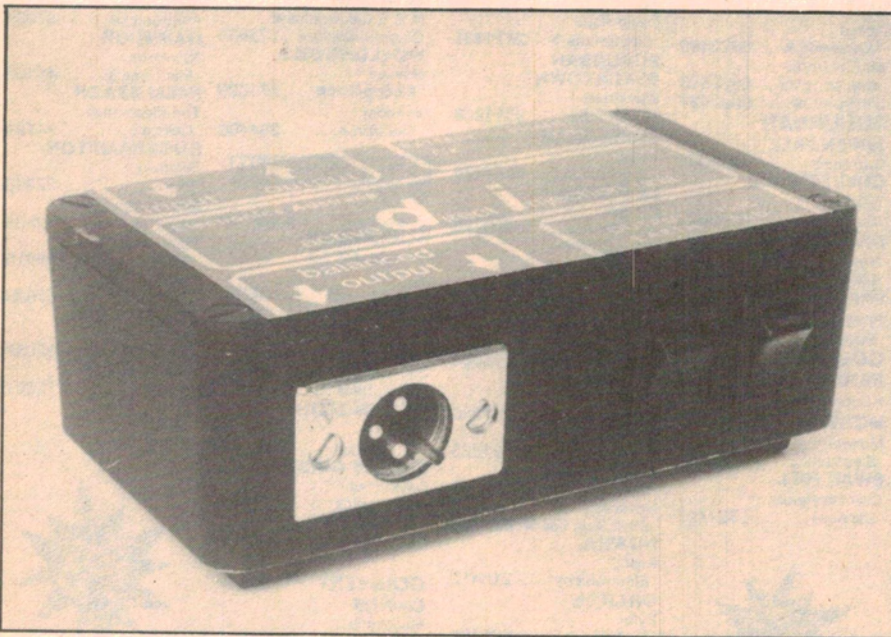
Designed for the rigours of professional use, the DI is housed in a diecast box and uses rugged flush mount switches.
