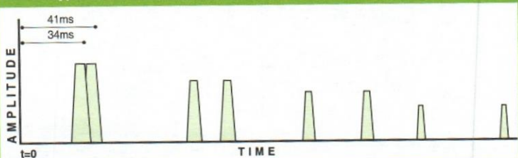
Type 4 Reverb Unit Output for Single Pulse Input at Time t=0
