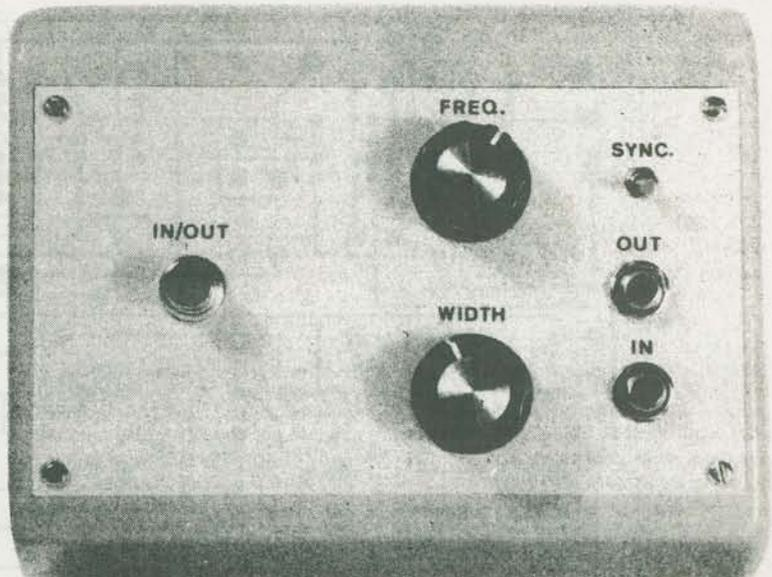
The finished echo unit, showing the footswitch mounted on the far left of the front panel.
