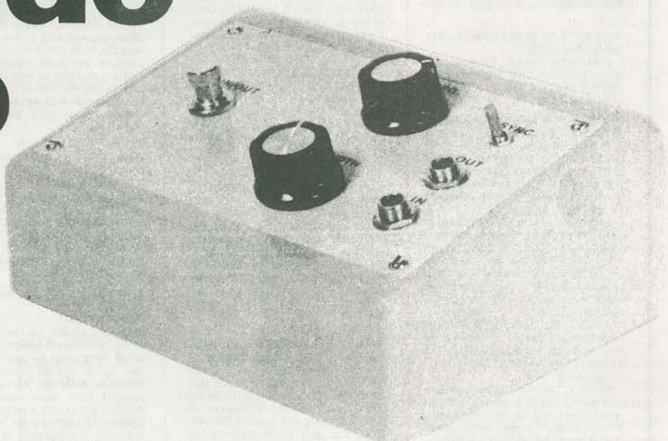
This device is really a form of tremolo unit, but when used with an instrument (such as a guitar) which has a fast attack and slow decay, it provides an effect which is much more like an echo effect than a conventional tremolo type. The unit differs from a standard tremolo rather than the more usual sinewave or triangular signal.
