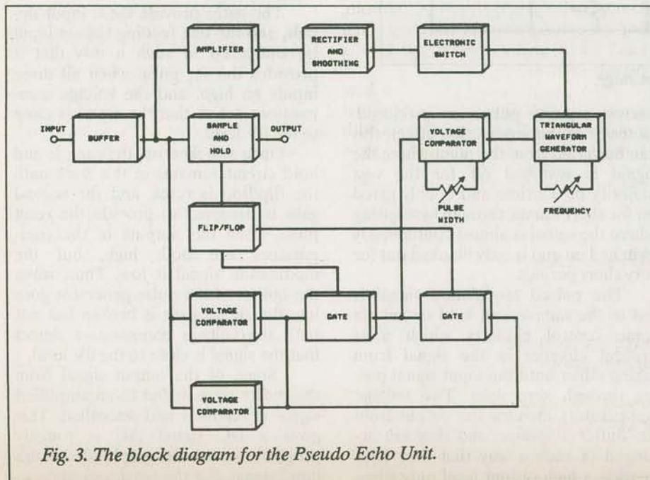
Fig. 3. The block diagram for the Pseudo Echo Unit.
