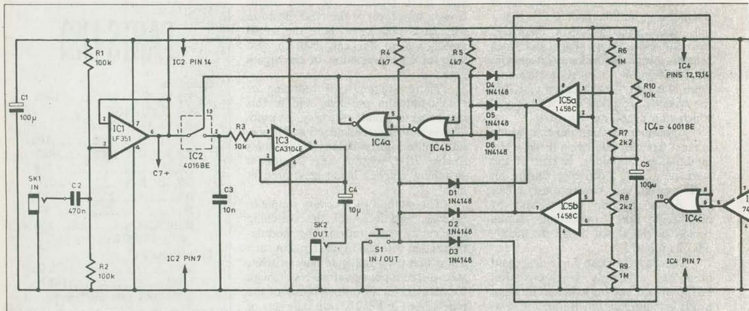
Fig. 4. The main circuit diagram for the Pseudo Echo Unit.
