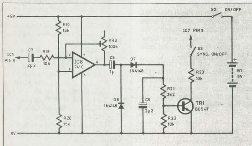
Fig. 5. Circuit diagram for the synchronization stage.
