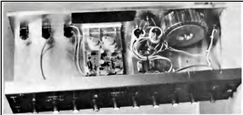
Completed wiring in chassis.
