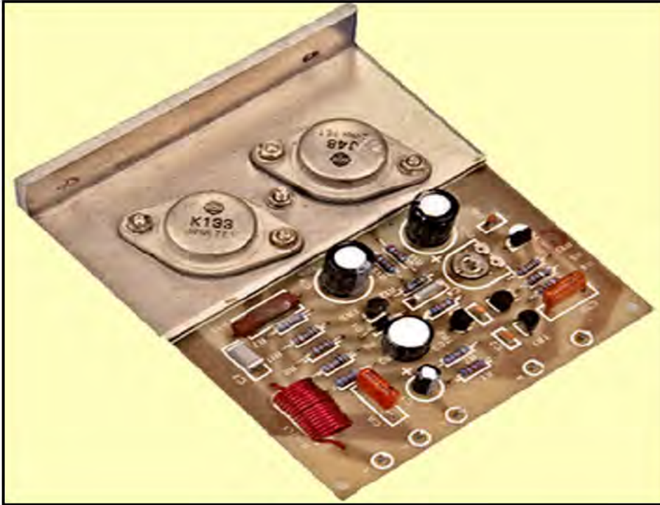
Completed MOSFET Amplifier.
